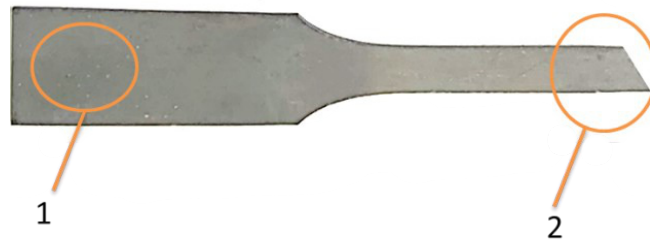
Fig. 9. Positions for measurement of hardness and microstructure observation
